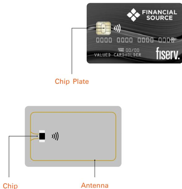
Contactless EMV cards include a more powerful EMV chip and an antenna, enabling fast and easy tap-and-go payments.
